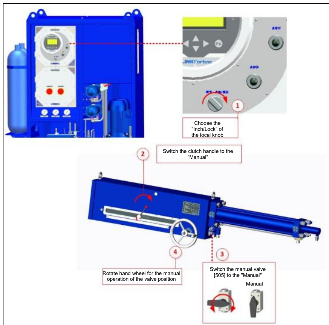
Figure 14: Site mechanical manual switching workflow of iSA controller oil pump
