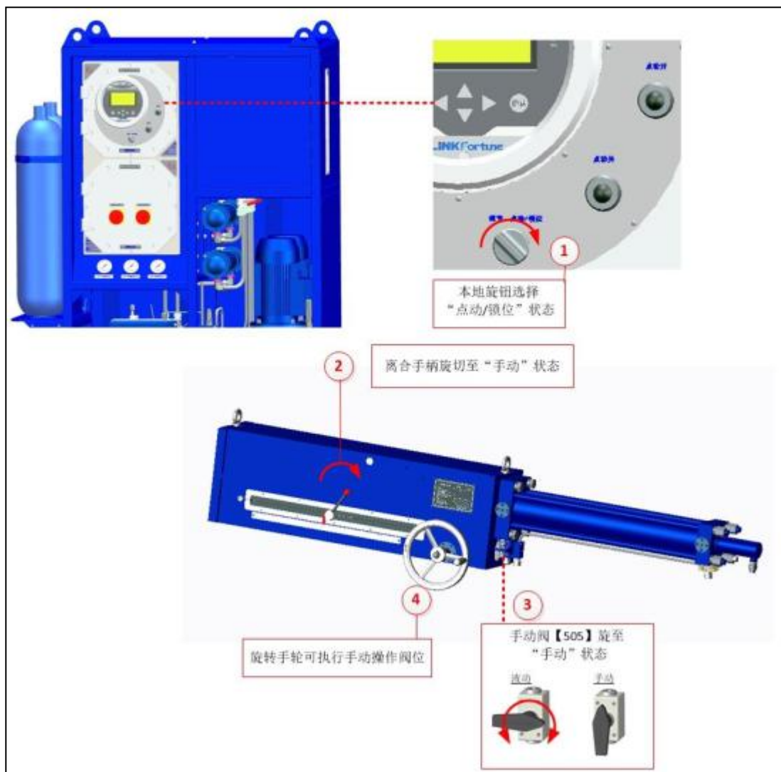
Figure 14: Site mechanical manual switching workflow of iSA controller oil pump (Continued)
